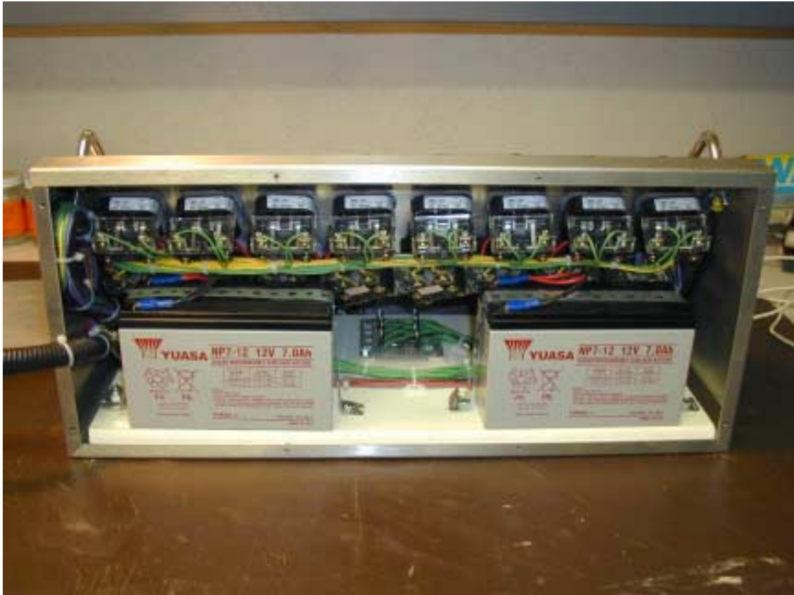
Inside view of console showing batteries
