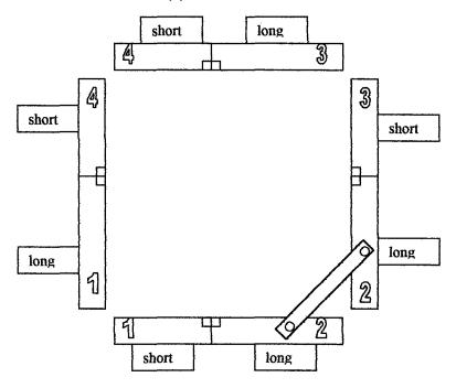
Place two frame sides together with the counter-bored sides facing each other and with matching corner numbers together.
