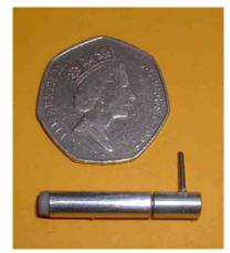
A few notes on construction. I learned only late in life that aluminum tubing can be cut cleanly by rolling a scalpel blade across it. Make the first revolution very carefully so that you have a continuous cutting line. Then work the blade to and fro until the component separates off. But beware! Small sections, such
