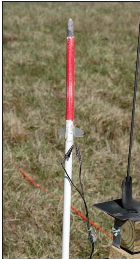
A Cheap and Easy Piston ready for launch. The igniter leads are bent to extend out of the top of the piston tube for simple hookup.
