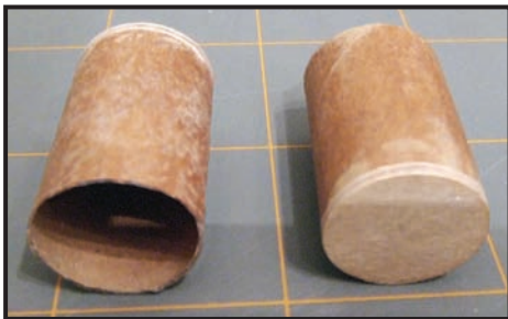
Two piston heads made from coupler stock and bulkhead disks.
