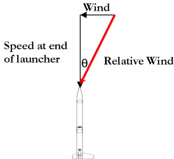
A 30 ounce, 2.6" diameter HPR design powered by an H180 reaches 45 mph from a 3' rod and 60 mph from a 6' rod.
