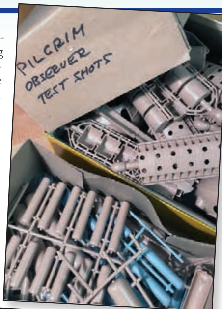
Test shots of the parts for the Pilgrim Observer plastic model kit.
