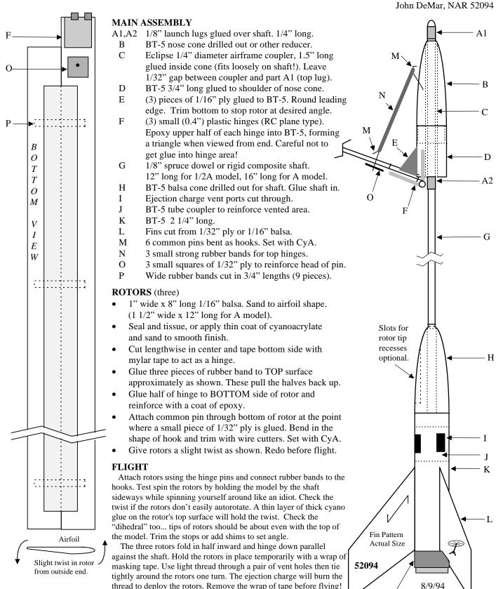
A launch tower is recommended (or add a launch lug at fin joint). Use 1/2A3-2T or A3-4T. Tape engine to body tube to hold it in.
