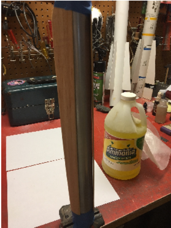
Blades Taped on Mandrel Before Wrapping
