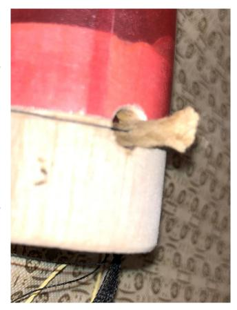
ends of the burn thread. knot on the opposite side of the shoulder from the fuse, and scure with a drop of CA glue. Trim the Pass the end of the burn string through the loops of the shroud lines and over the leash line. Tie a
