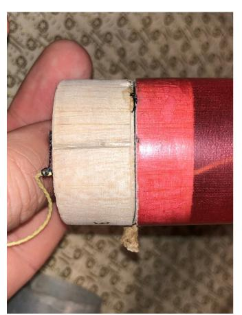
Aligh the notch in the body tube with the DT fuse and seat the cone on the model. you to keep the shock cord and shroud lines under control as you insert the shoulder into the tube Pack your chute as usual, making sure to avoid tangles. The grooves in the shoulder should allow
