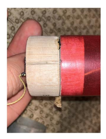
inner surface of the shoulder. below where the nose cone ends to hold the burn string. Two notches are made to hold the shoud notches in the base of the nose cone and the top of the body tube. A small groove is carved just There is a hole drilled in the shoulder to hold the fuse. A hole punch is used to make corresponding lines (wide and shallow) and the shock cord (narrow and deeper). The shock cord is glued to the
