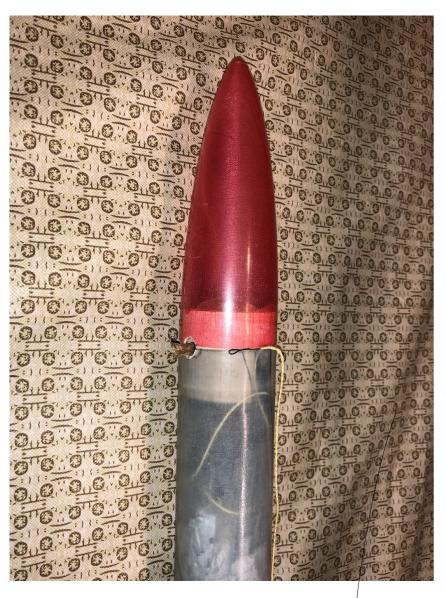
Jordi carves a hollow balsa wood shouler to hold the fuse, release string, and shroud lines together. I can't think of a reason why a foam shoulder couldn't be used.
