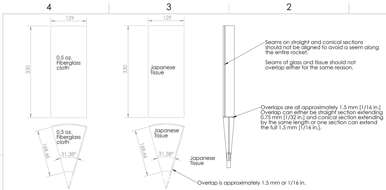
Configuration #2 One layer of fiberglass and one layer of tissue
