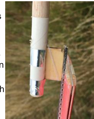
Two side views of the burn thread routing. The thread is taped on the body tube in a "U" so that it won't slip.
