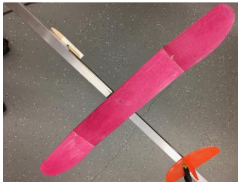
Aluminum angle clamped to the tail can align the power pod pylon during assembly.
