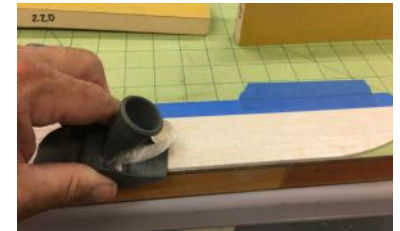
A razor plane makes quick work of roughing out the airfoil.
