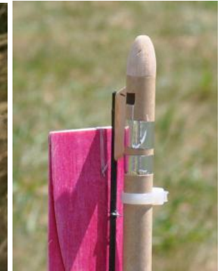
Two side views of the burn thread routing. The thread is taped on the body tube in a "U" so that it won't slip.
