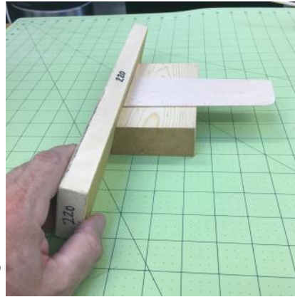
Homemade sanding block and bevel jig. Jig is simply a pine block cut with an 8 or 10° angle on one face.
