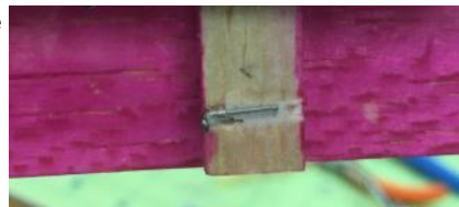
Using a square block and a small button magnet to align the fin for gluing.
