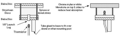
up a shield for the thermistor to protect it from sunlight. One kind of shield is shown in Figure 8 and is made from wood and styrofoam (foam 3/16" thick from a meat tray). The top disc is larger to help
