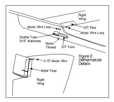
The D-Light's D/T design is shown in Figure 2 above. The flap is cut out after the wing is installed on the glider, then a piece of fine (.015 inch) music wire is bent in a Z-shape, with one of the ends then being glued (with cyanoacrylate glue) to the main wing and the other (which is bent upward by 30 degrees or so) to the wing flap while it is in the raised
