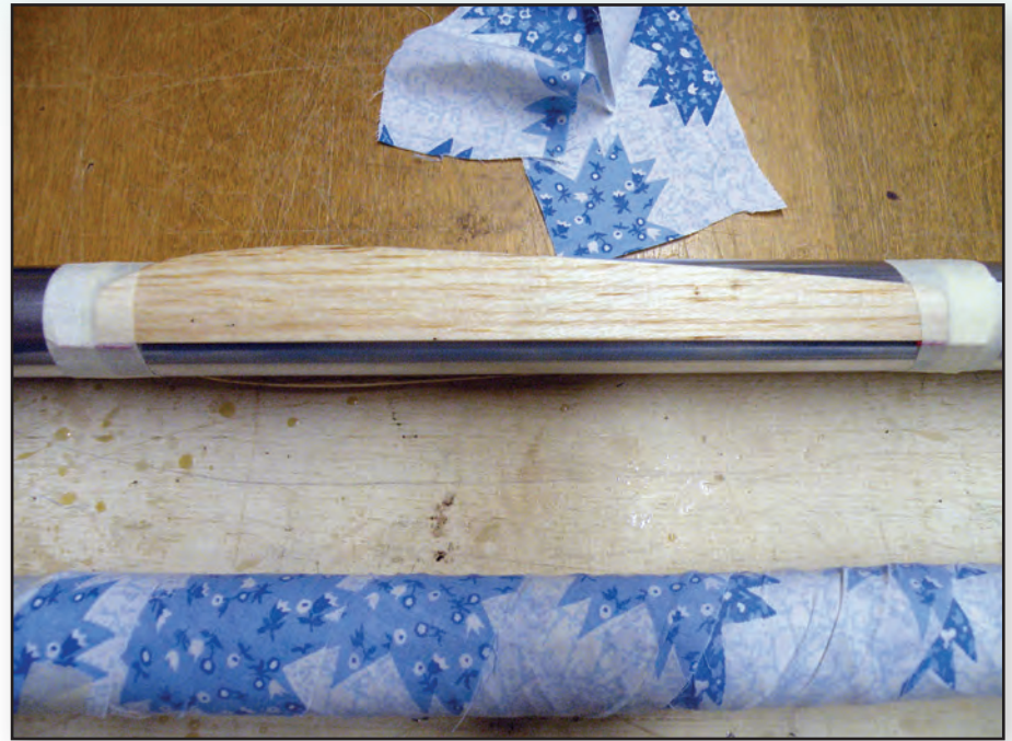
Photo 3. Wet S9 blades taped to mandrel (top) and wrapped with cloth strips (bottom).
