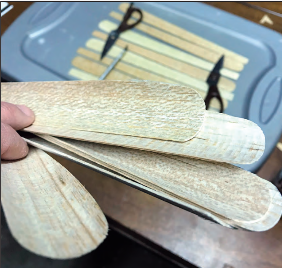
Photo 4. Set of dry S9 formed blades (with some more soaking in ammonia solution in background).
