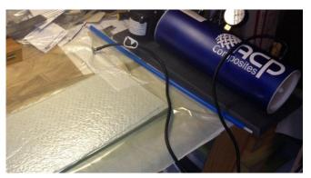
limit switch such that the vacuum pump does not need to run continuously. The ACP Auto-Vac system is very convenient but not cheap. A variety of lower price options can be found on the internet.
