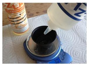
Be sure to accurately measure the resin and hardener amounts. Using a scale accurate to 0.1 grams is recommended. After pouring the resin and hardener, be sure to stir very thoroughly.
