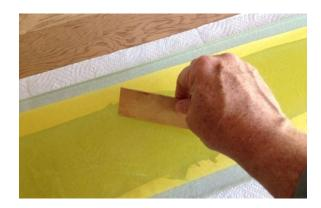
squeegee to remove any excess epoxy from the laminate. Remember that the strength of the laminate comes from the plies, so excess epoxy only adds unnecessary weight. You'll quickly get a feel for how much pressure to apply to remove excess resin.
