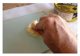
The layer of wax might be sufficient release treatment. However, to be prudent, apply a layer of release agent. Spray-on release (such as LPS MRX silicone mold release<sup>7</sup>) provides a smooth uniform finish. Liquid release (such as FibRelease<sup>8</sup>)might also be used. If using liquid release, allow the release material to dry before proceeding with the layup.
