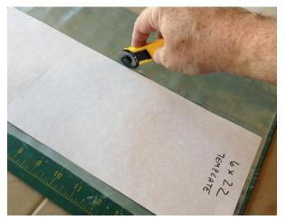
the correct size in a repeatable manner. You should also use a composite cutter and cutting mat to easily cut fiberglass and carbon veil. Use scissors to cut breather cloth. Scissors or razor blades are best for cutting release ply.
