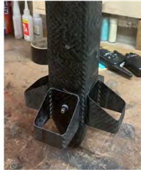
Prototype #2 2.0" x 2.0" tube fins at base of booster
