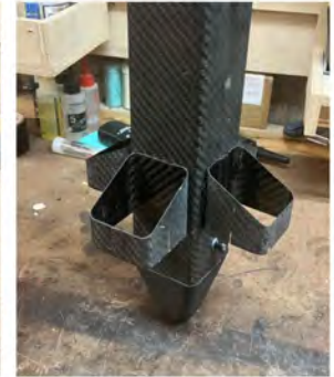
Prototype #3 2.0" x 2.0" tube fins 2.5" up from base of booster
