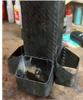
Prototype #1 1.25" x 2.5" tube fins at base of booster
